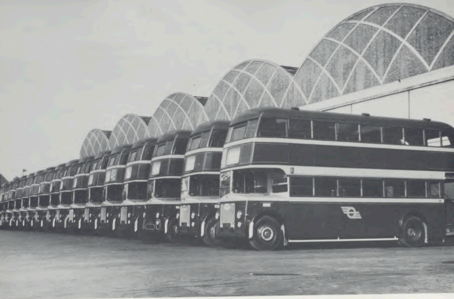
Some of the new 74 seater buses, with fully automatic transmission, outside Donnybrook Garage.
