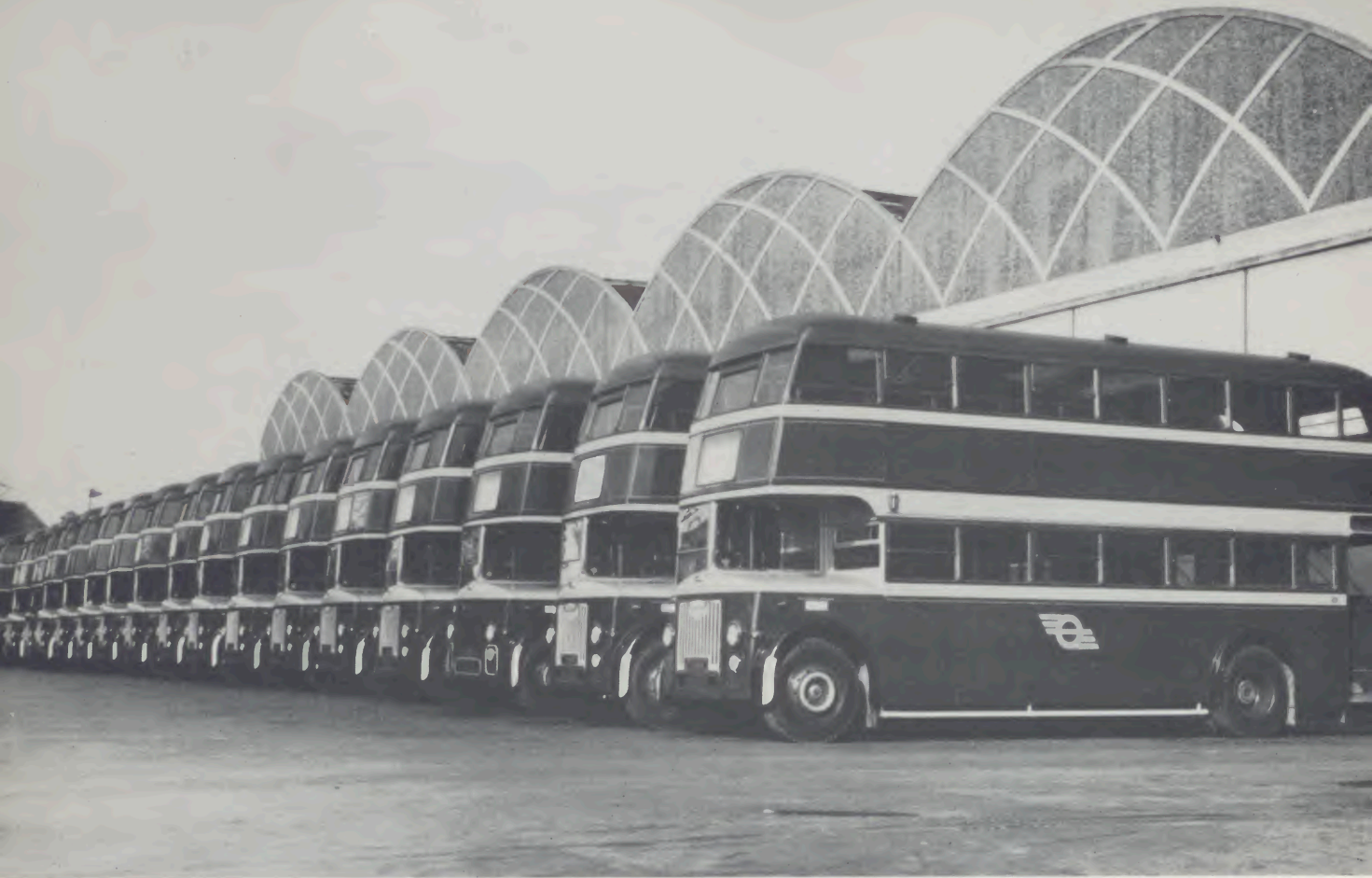
Some of the new 74 seater buses, with fully automatic transmission, outside Donnybrook Garage.
