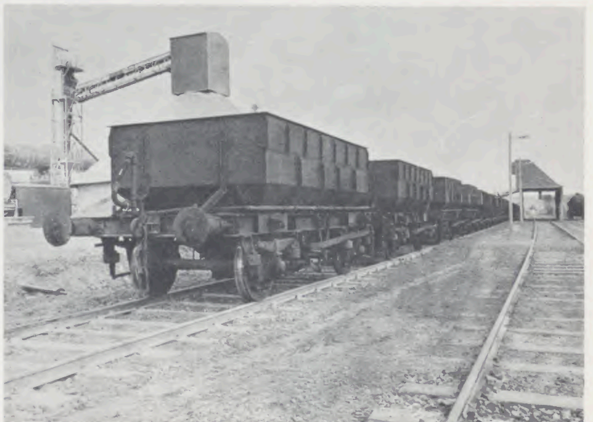
CIE bulk ore traffic continues to increase and special wagons have been designed and built by CIE and C. A. Parsons of Ireland Ltd.
