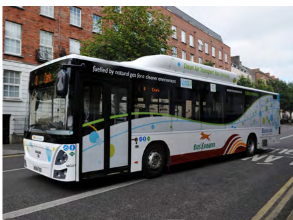
In 2012, Bus Éireann introduced the first trial in Ireland of a Compressed Natural (CNG) Gas public transport vehicle.
