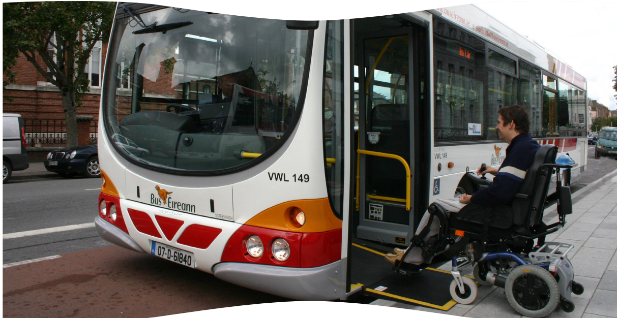
One of the new Transport 21 low floor accessible city buses.
